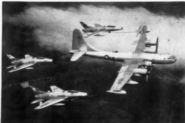
KB-50 REFUELS three F-100s at once using probe-and-drogue in tests at Eglin AFB.
